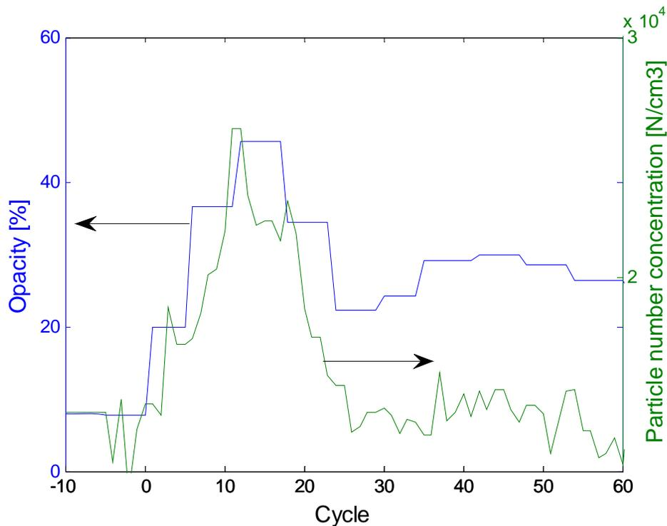
**Figure 15** Variations in mass-averaged particle diameter during a transient can be estimated by comparing opacity and particle number measurements.
