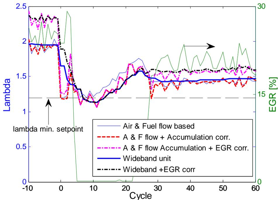
**Figure 12** Correction of the estimated air/fuel ratio
