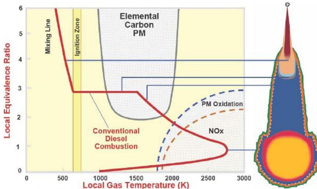
**Figure 6** Emission formation in conventional diesel combustion, [8].
