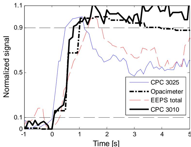
**Figure 13** Rise time evaluation for PM instruments
