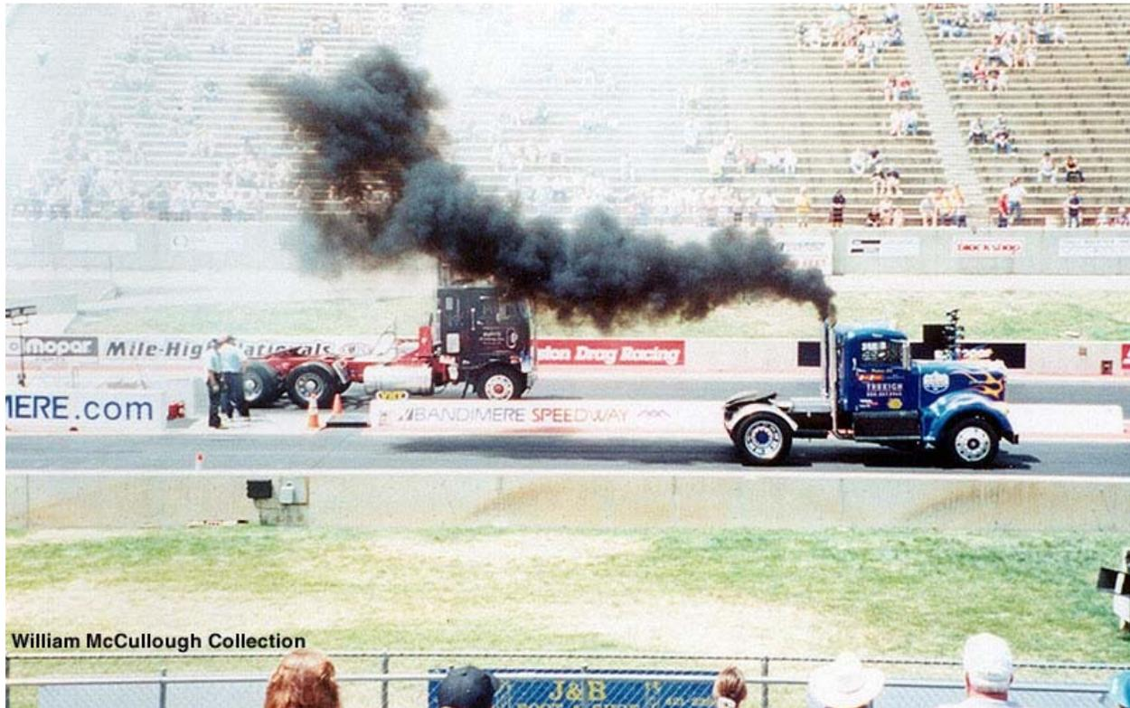
**Figure 5** Soot can be an issue during acceleration [7]
