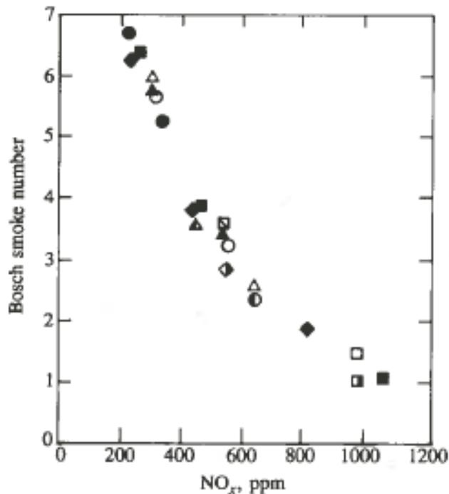
**Figure 7** Example of a soot-NO<sub>x</sub> trade off curve. [9]
