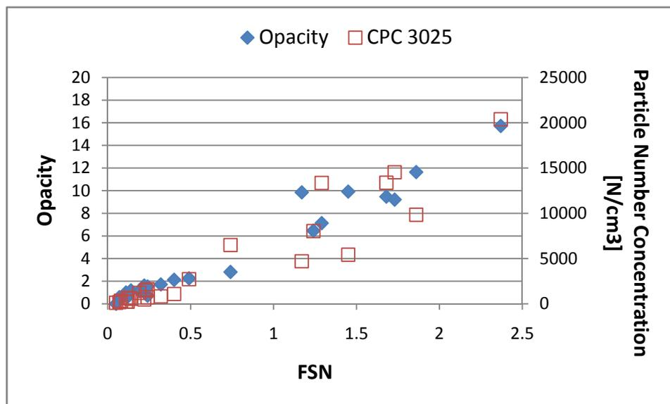
**Figure 14** Correlation between PM-measurement methods
