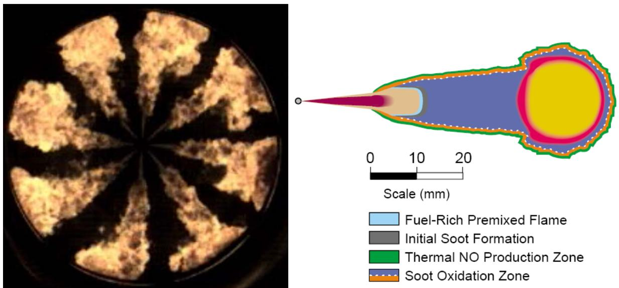
**Figure 2** Diesel combustion process, [3], [4]
