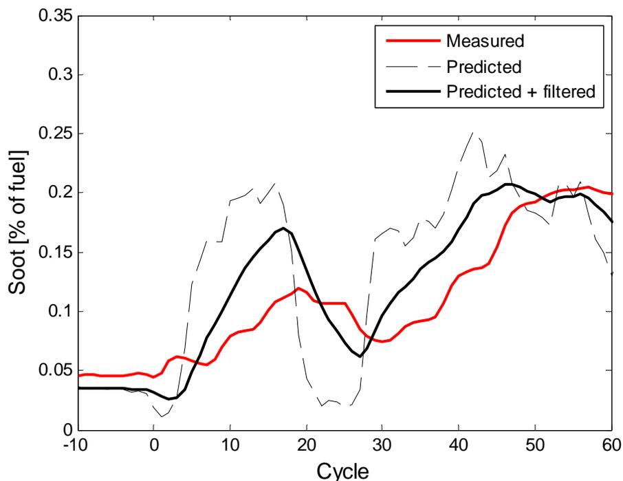
**Figure 15** Post processing of predicted soot emissions to imitate exhaust system and instrument averaging and to decrease effects of noisy input data.
