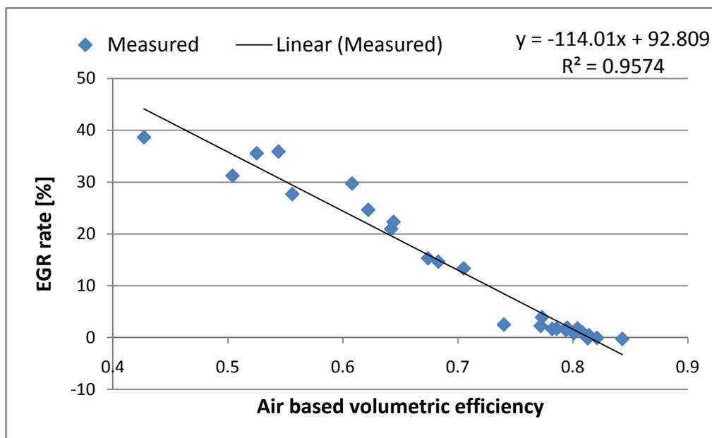
**Figure 11** Steady state correlation between air based volumetric efficiency and EGR rate for a wide range of operating conditions
