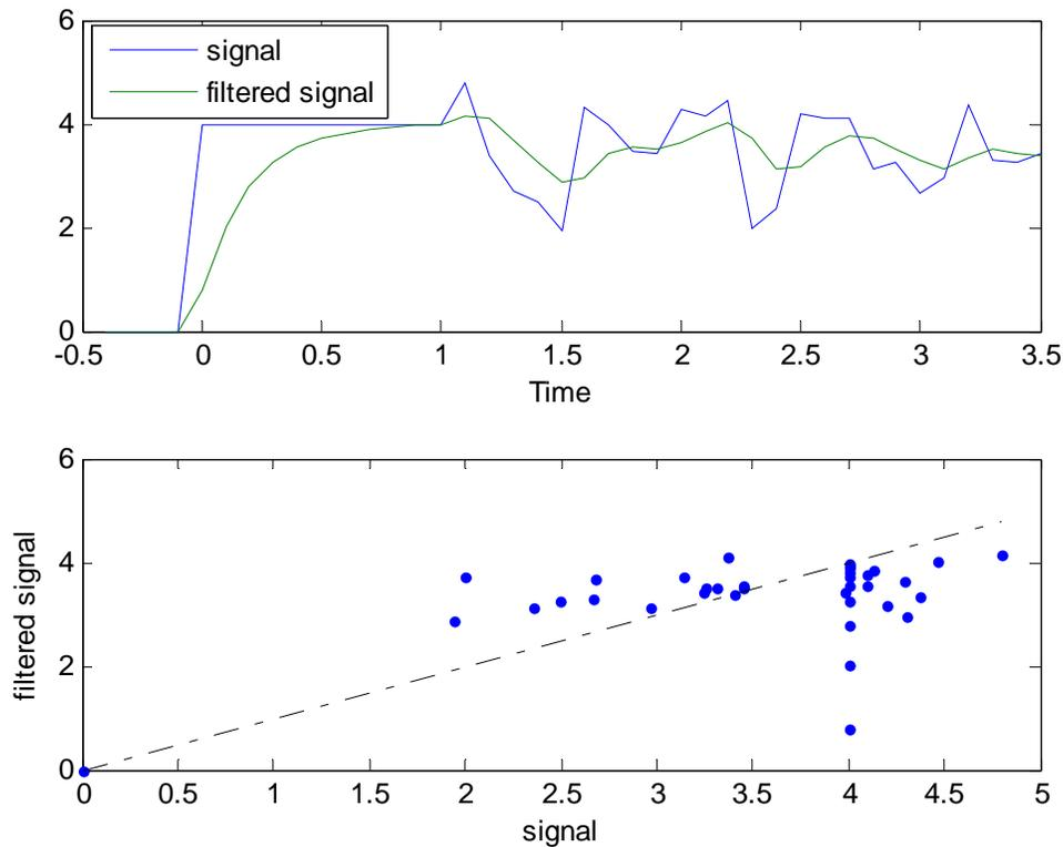
**Figure 10** Effects of instrument rise time on statistical models.
