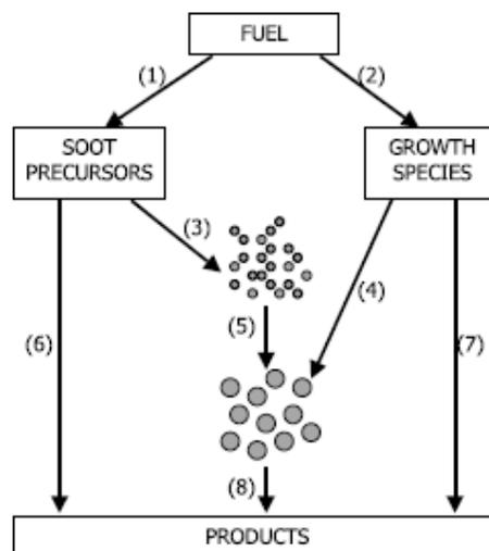
**Figure 9** Illustration of Fusco et al's Soot model [17]. Schematic figure from [25]
