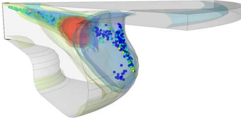
**Figure 7** CFD Modeling of the diesel combustion process [12]
