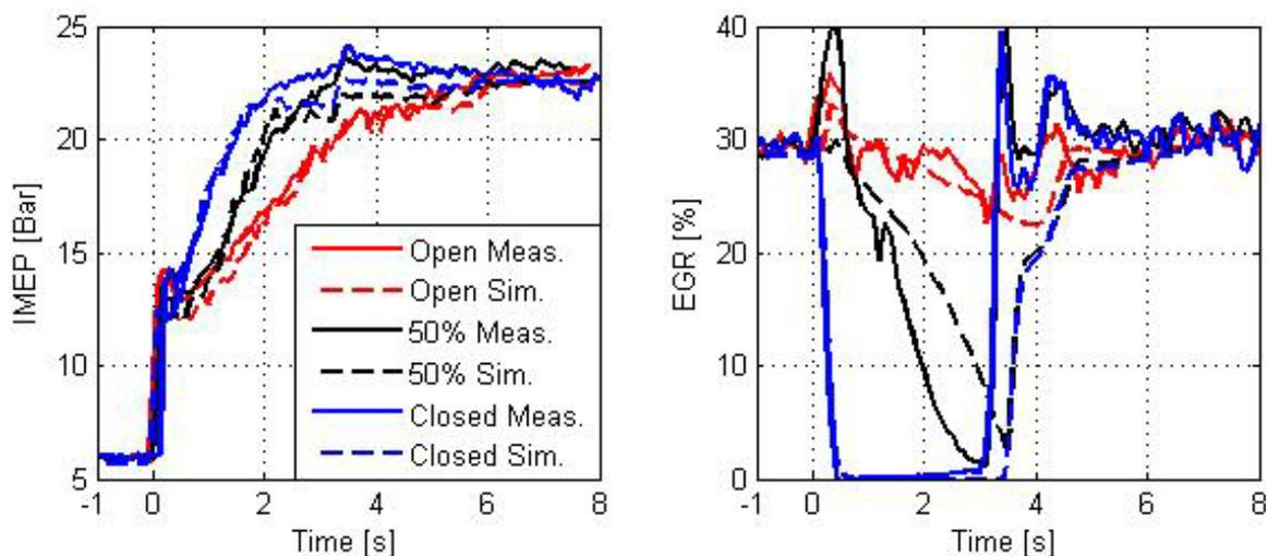
**Figure 16** Predicted and measured IMEP and EGR rate with three different EGR-valve settings during the initial part of a transient.
