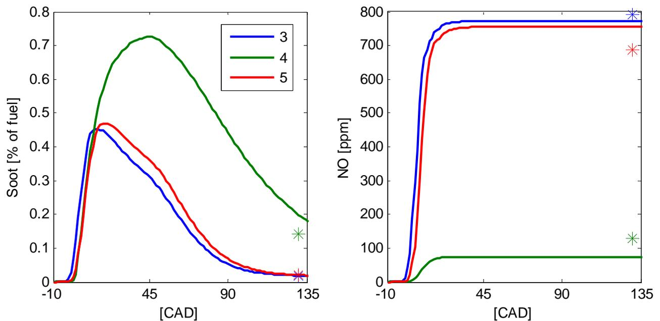
**Figure 17** Crank angle resolved emission predictions. Case 3 and 5 are identical besides regarding injection angle. Case 4 and 5 are identical besides regarding EGR rate. The stars (\*) show the measured values for the different cases.
