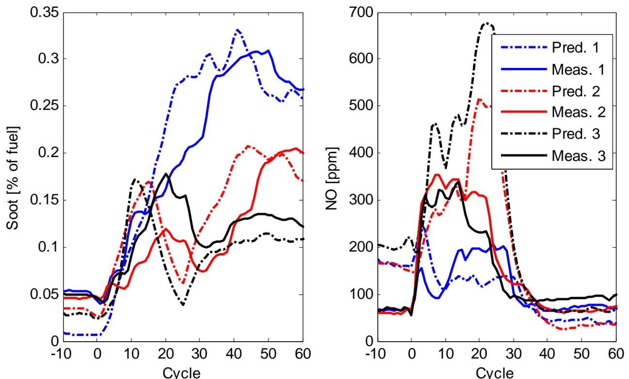
**Figure 18** Predicted emissions during a load transient with three different strategies. The strategies are identical in case 1 and 2 besides the EGR-valve position during the first 10 cycles. Case 2 and 3 are identical besides the VGT position during the first 20 cycles of the transient
